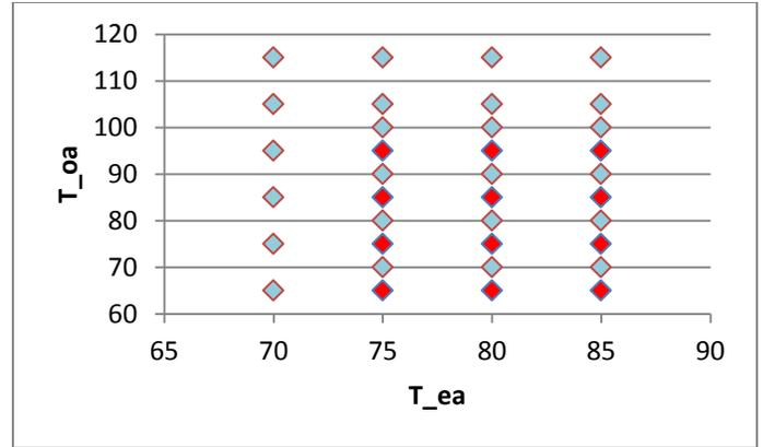
**Figure 4: Map of test conditions used for parameter identification (red) and model validation (grey). The axes are outside air temp (°F, vertical axis) and evaporator air temp (°F, horizontal axis).**
