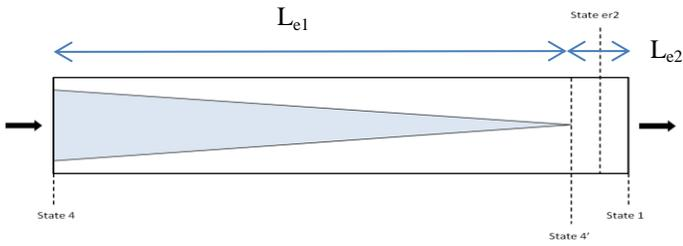
**Figure 3: Conceptual model of the evaporator, showing saturated and superheat regions.**
