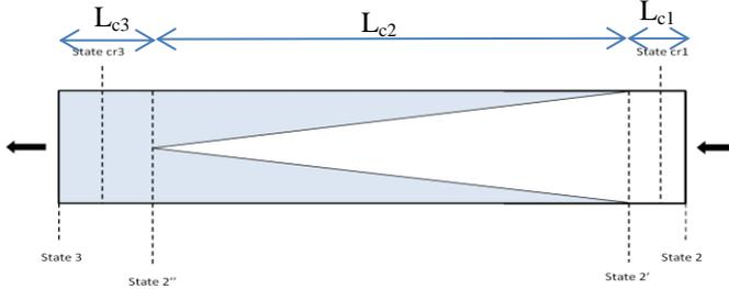
**Figure 2: Conceptual model of the condenser, showing superheat, saturation and subcooled regions.**
