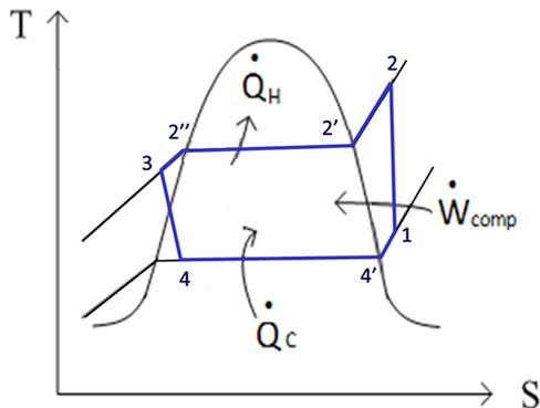
Figure 1: Temperature-Entropy Diagram of the VCC showing condenser sub-cool and evaporator superheat.
