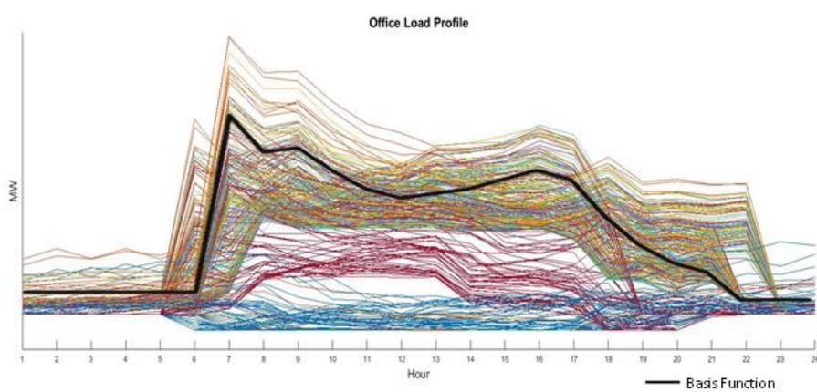
**Figure 1:** Basis Function for commercial load.
